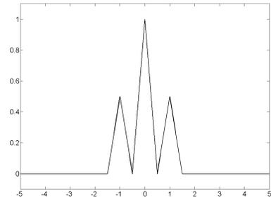
Fig. 3. Autocorrelation for example  $s$  in figure 1, which is not monotonic on  $t \geq 0$
