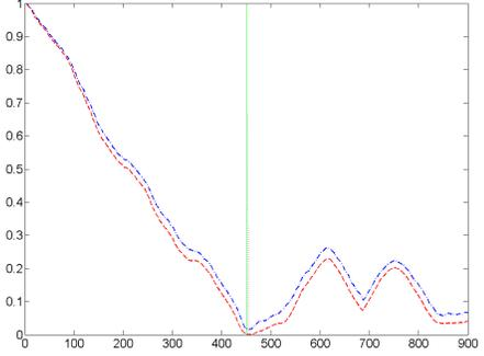
Fig. 7. Discrepancy correlation coefficient and its  $\Gamma_p$  approximation with  $p = 128$  for the reference patch of Figure 5; the upper curve refers to the approximation. Both curves show a well formed minimum around the correct position at 450
